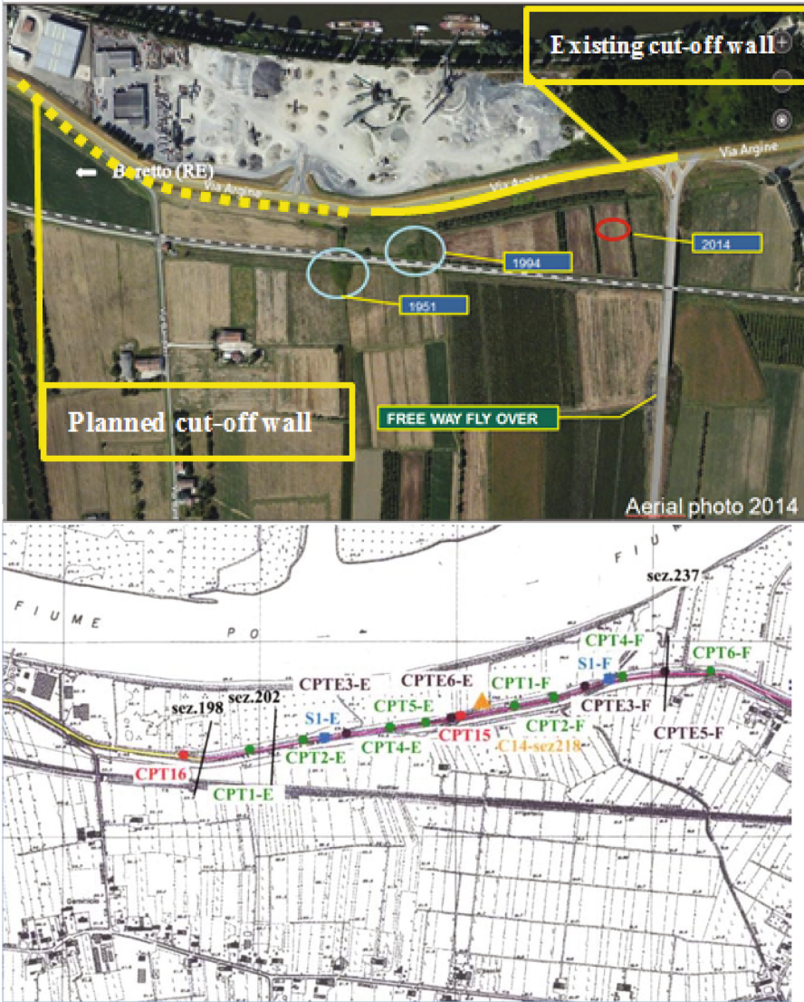
Fig. 7. Boretto: above: chronological order of the events where evidence from the 1951 and 1994 sand boil “cup” is visible; below: location map of the study area showing the borehole locations and interpreted profiles; S1-E/F = boreholes.
