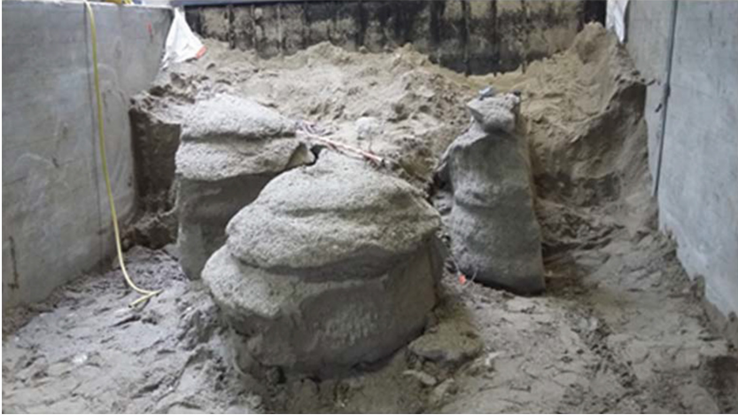
Fig. 7. Calcified block after excavation in 0/4 mm sand, above the gravelly foundation (test B1)
