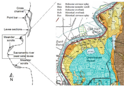
Fig. 2. Sacramento River Levee system in California showing a clip of a geological map with most common geomorphic features
