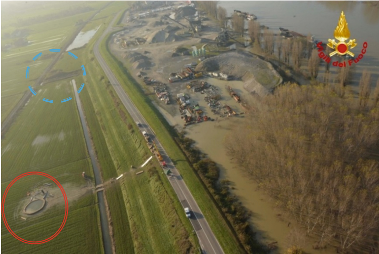
Fig. 8. Boretto: the 2014 flood induced sand boil (red double line circle) at about 70 about 320 m downstream from a previous sand boil “cups”, dating to 1951 and 1994 (light blue dashed line circle).
